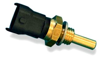
This sensor is designed to measure fluid temperatures e.g. oil, water or fuel. This signal may be used as a control value for engine control units or as a measurement value which is logged in a data acquisition system.
