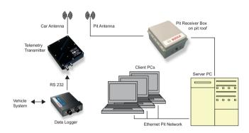
The Bosch Motorsport Online Telemetry System enables the transmission of online measurement data from a car on a racetrack. The vehicle part of the system consists of a data and the FM 40 telemetry transmitter. From the data logger data is sent via a RS232 connection to the FM 40. The FM 40 adds framing and error correction information to the data stream and modulates its RF output which is fed via an antenna wire to the TX antenna.
