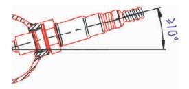
Recommended design of the mating thread in the exhaust pipe \*: THexagon > 600°C or TGas > 930°C
